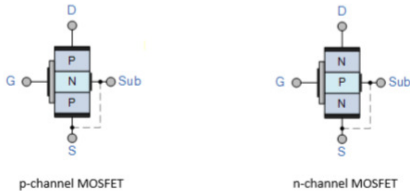
Figure 7: Illustrate the p-channel and n channel in MOSFET.
