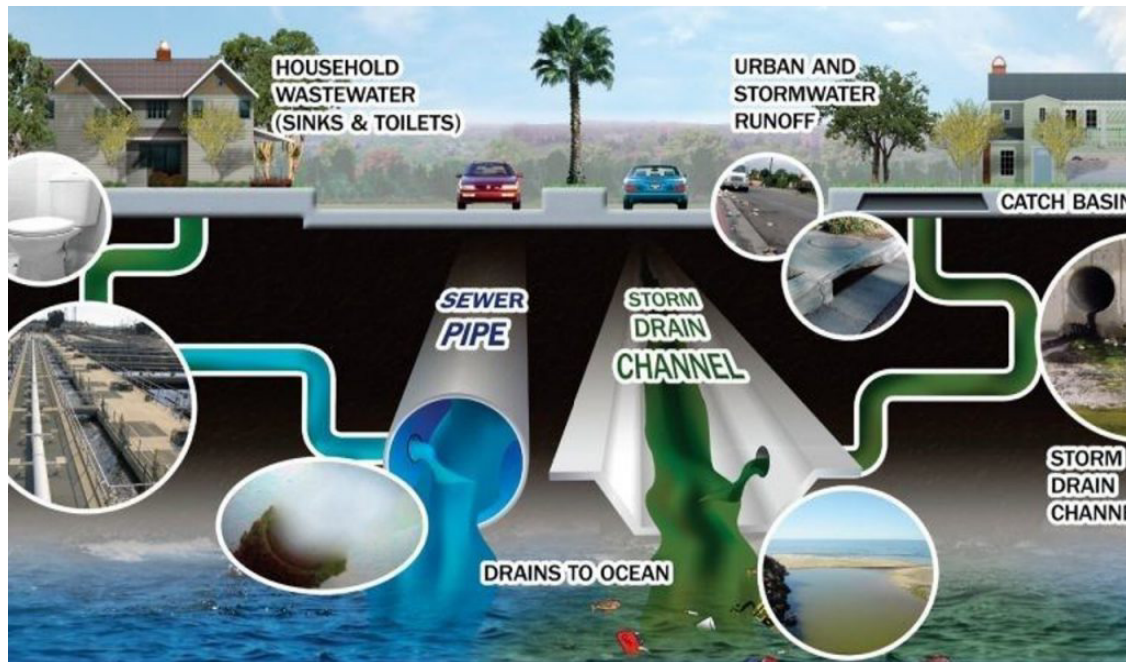
Figure 4: Illustrates the Stormwater Prevention Method.
