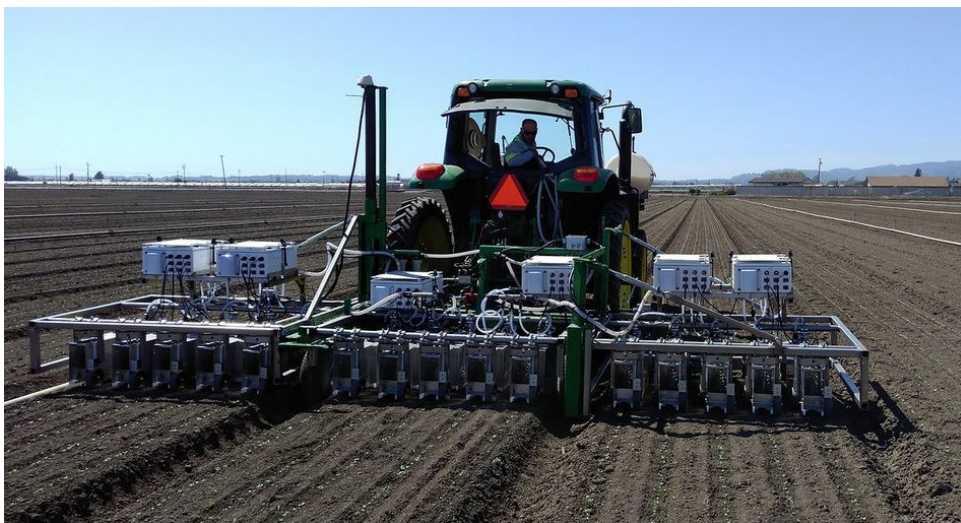
Figure 6: Illustrates the Vision Robotics. The Vision Robotics range of robots can automatically thin plants, especially lettuce, and prune vineyards. It is sophisticated with its AI-powered mechanisms [Source: Wevolver].
