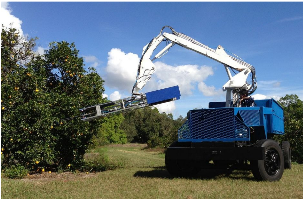
Figure 4: Illustrates the Energid robot which is mainly utilized for assisting the growers in plucking the citrus fruits from the farm. It can pluck one fruit in 2-3 seconds, and the overall cost is cheaper than human labor [Source: Wevolver].
