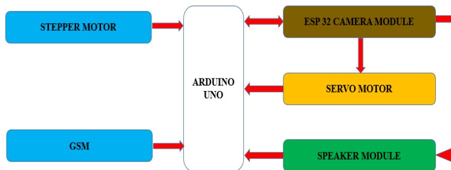
Figure 2. Illustrate Block Diagram of Smart Security System for Enhancing Security for Home and Office.
