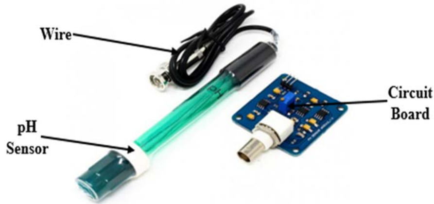
Figure 3: Represents the pH Sensor Kit for Analyzing the pH of Soil [9].
