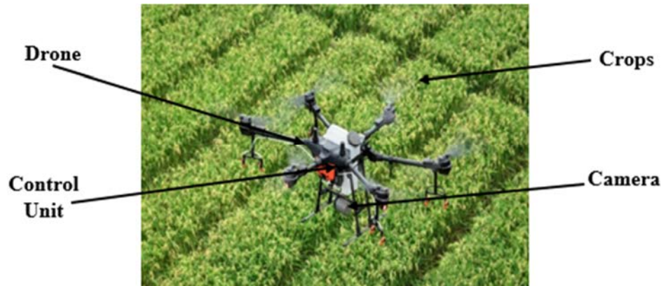
Figure 1: Illustrates the Aerial Surveillance Vehicle for the Agriculture for Analysis of the Conditions of Crops in the Soil [4]
