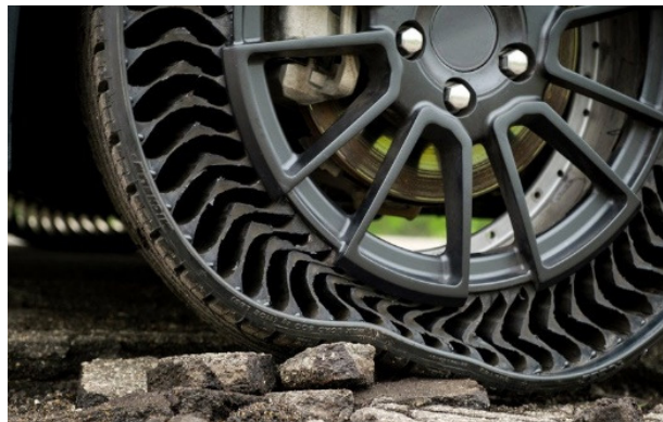
Figure 2: Representing the puncture-proof and Airless tire with the Support of AM [10].
