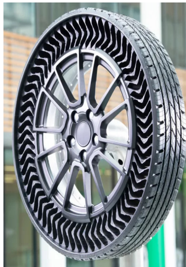
Figure 2: Showing Michelin Tweel's design [17].
