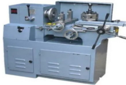
Figure 4: Represents Capstan Lathe Machines Used in the Industry for Different Machining Processes [17].
