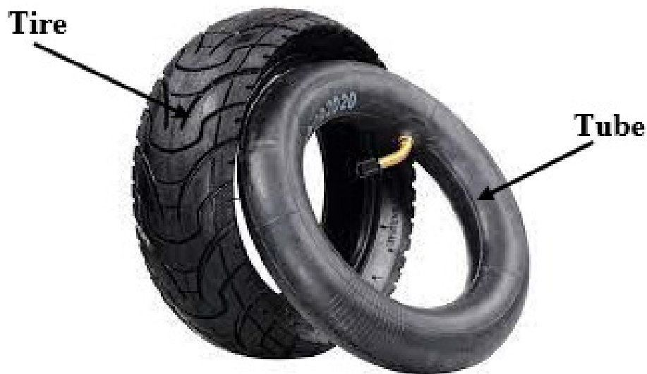
Figure 1: Represent the Tube Tire Arrangement of the Wheel of Four-Wheeled Vehicle.
