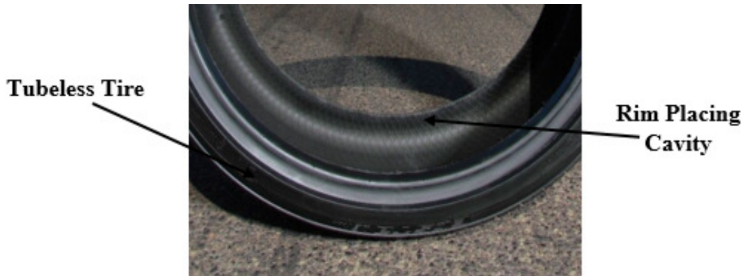
Figure 2: Represent the Tubeless Tire Wheel of a Two-Wheeled Vehicle [17].
