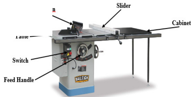
Figure 5: Represents the Design of the Cabinet Type Table Saw Used for Various Cutting Operations.
