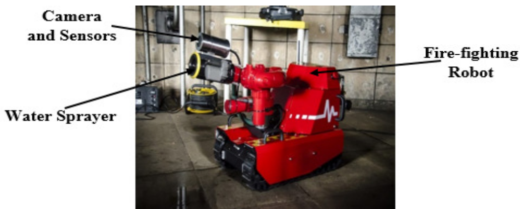
Figure 2: Represents the Firefighting Robots used for Fire Extinguishing Operations without Human Intervention.
