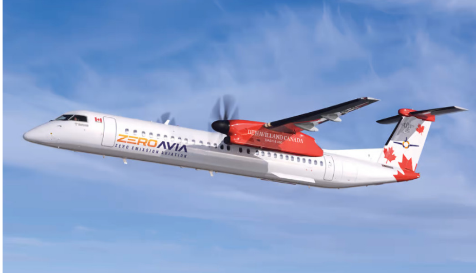
Figure 3: Represents the Flight of ZERO AVIA Which Uses Hydrogen as a Fuel to Achieve the Zero Emissions [7].
