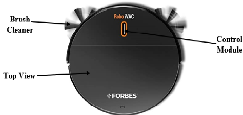
Figure 3: Represents the Robotic Cleaning Device for Automatic Clear of the Floor without Human Intervention.
