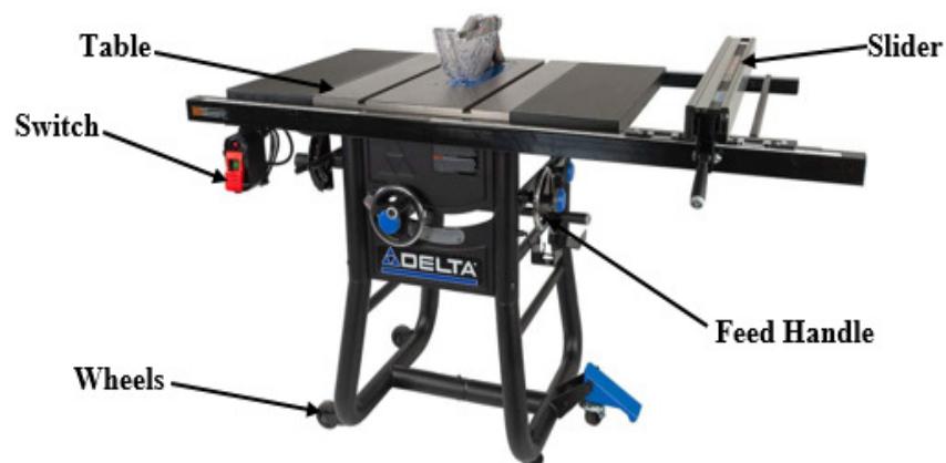
Figure 4: Represents the Design of the Jobsite Type Table Saw Used for Various Cutting Operations.
