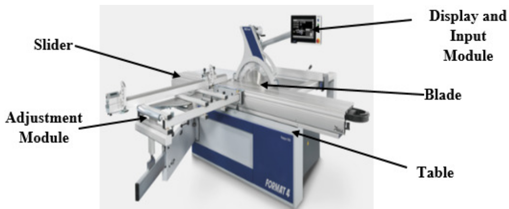
Figure 8: Represents the Design of the Sliding Type Table Saw Used for Various Cutting Operations [13].
