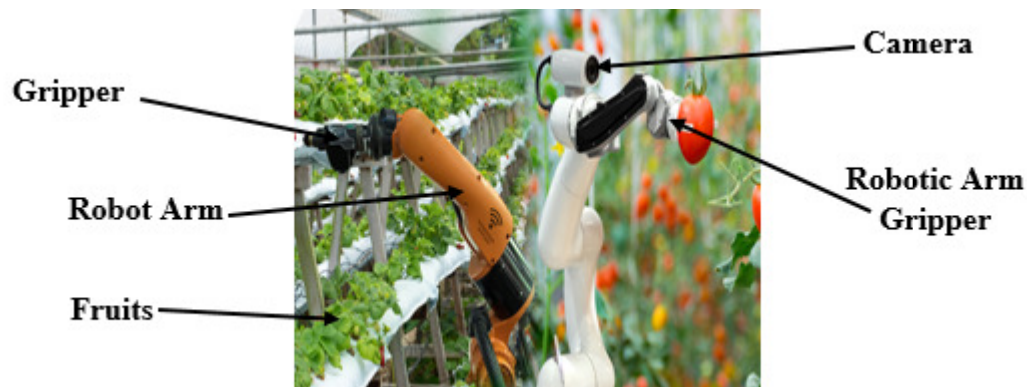
Figure 2: Represents the Working of Fruit Plucking Robots used in Various Agricultural Activities[8].
