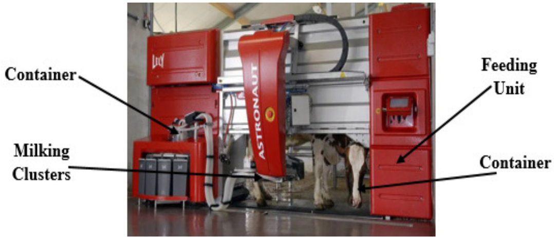
Figure 3: Represents the Milking Robot Setup in the Cattle Farm for Milking the Cows with Complete Automation.
