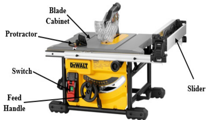
Figure 3: Represents the Design Of a Compact Type Table Saw Used for Various Cutting Operations.
