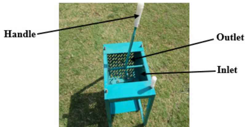
Figure 4: Represents the Manual Groundnut Shell Removing Machine for House or Domestic Use.
