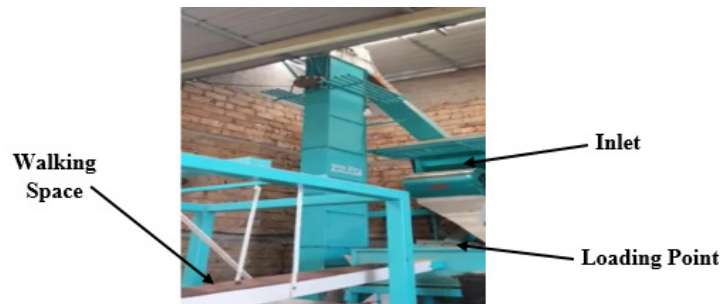
Figure 1: Represents the Automatic Groundnut Shell Removing and Collecting Plant in the Factory.
