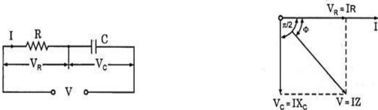
Figure 7.4: Resistance Capacitance (R-C) Series Circuit Diagram and Phasor Diagram
