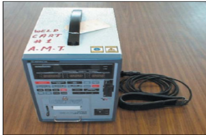
Figure 1 Rogowski-Type Current Sensing Coil and Meter Combination
