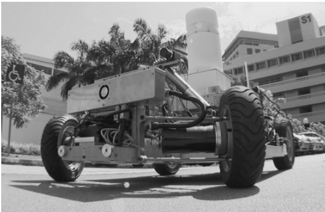
Figure 1: A 360° scanning MMW RADAR mounted on a vehicle test bed for SLAM experiments within the NTU campus [Lag Out].
