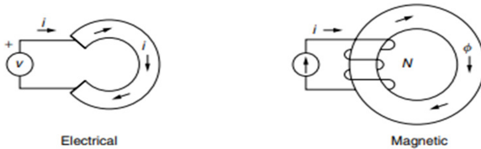
Figure 1.7: Show the circuit diagram of electrical and magnetic circuit
