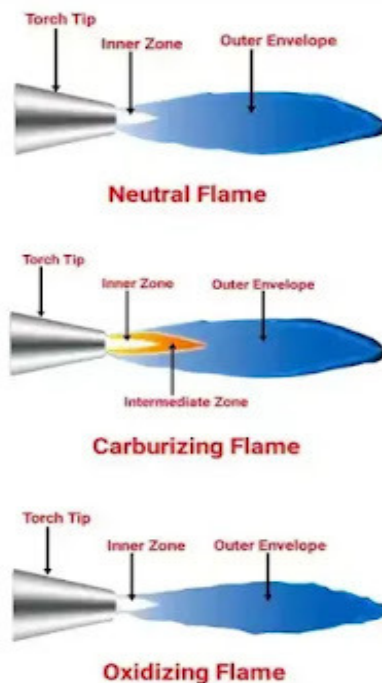
Figure 1: Representing the type of gas welding flame [Mechanical].
