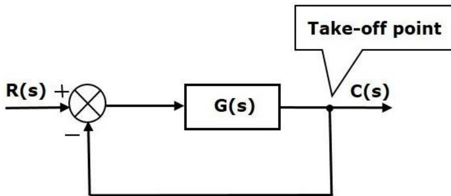
**Figure 5.5:** Illustrates the output  $C(s)$  are connected to the take-off point in the accompanying diagram as being one of the inputs to the summing point.
