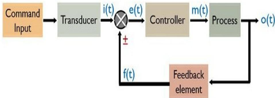
**Figure 2.2: Illustrates the comprehensive block diagram depiction of a closed-loop control system.**
