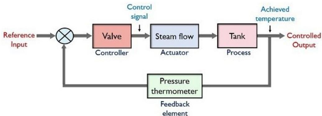
**Figure 2.3: Illustrates the block diagram depiction of a closed-loop system.**
