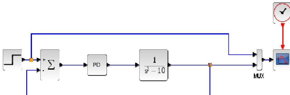
**Figure 6.14:** Illustrates this system can be brought from being unstable to being marginally stable.
