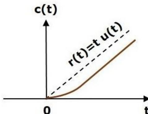
**Figure 8.10:** Illustrates the figure below is the unit ramp response.
