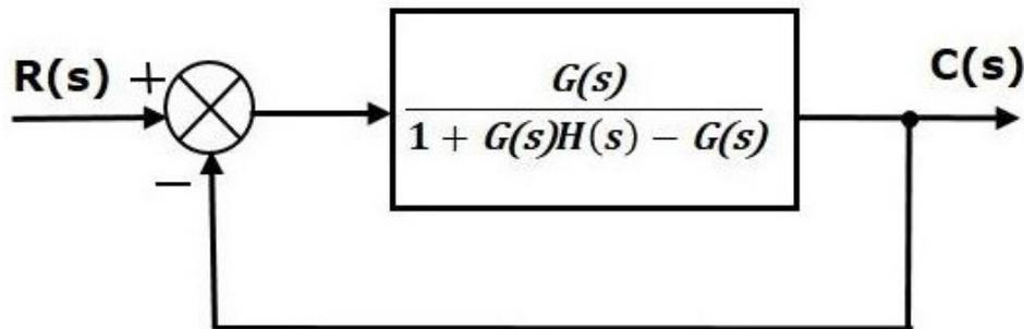
**Figure 9.5: Illustrates the leaving the unity negative feedback in its current state.**
