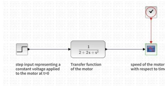
**Figure 5.1: Illustrates the step wise modelling of transfer function.**
