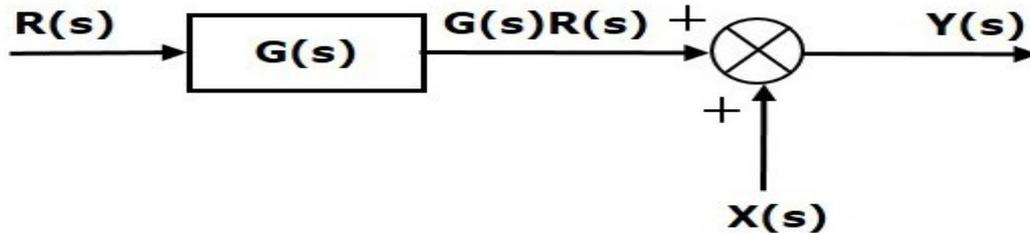
In both equations, the initial term,  $G(s) R(s)$ , remains the same. But the second term differs from the first. Only need one more block  $1/G$  to get the second term to be the same ( $s$ ). It has the input  $X(s)$ , and its output is used as the input to a summing point in place of  $X$ . ( $s$ ). The next figure displays this block diagram.
