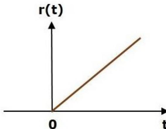
**Figure 8.6: Illustrates the unit ramp signal.**
