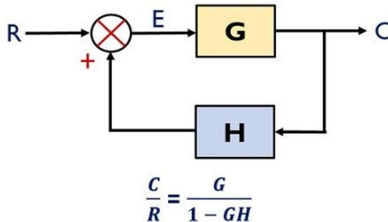
**Figure 1.6:** Illustrates the positive feedback loop with input output signal.
