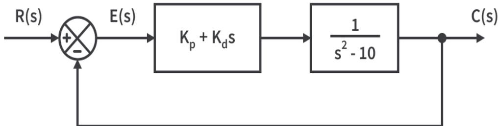
**Figure 6.15: Illustrates the derivative control will be added since they need to dampen the oscillations in this situation.**
