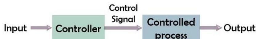
**Figure 1.9: Illustrates the block diagram of an open-loop control system.**
