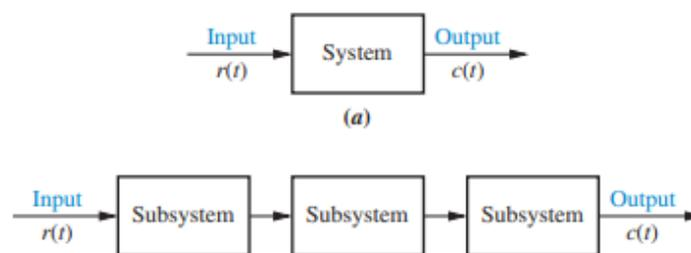
**Figure 3.1:** Illustrates the connection between the input and output of a system.
