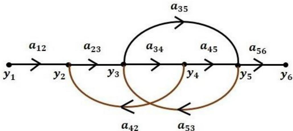
Block diagrams are transformed into signal flow graphs.
