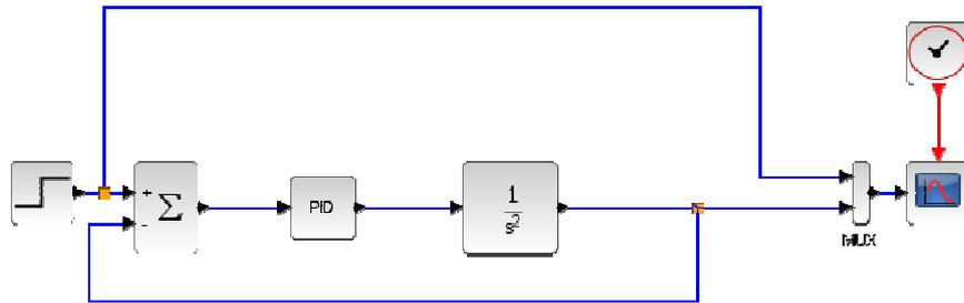
**Figure 6.12.** This system is totally oscillatory regardless of the value of  $K_p$  since it is only moderately stable (has poles just on imaginary axis) for just a step input.
