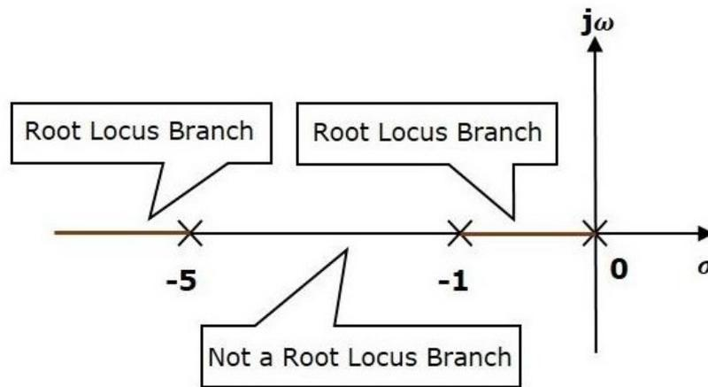
**Figure 10.2:** Illustrates the number of root locus branches is equal to the number of poles of the open loop transfer function.
