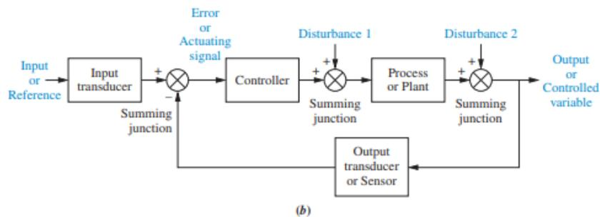
**Figure 2.6: Illustrates the configuration of open closed system.**
