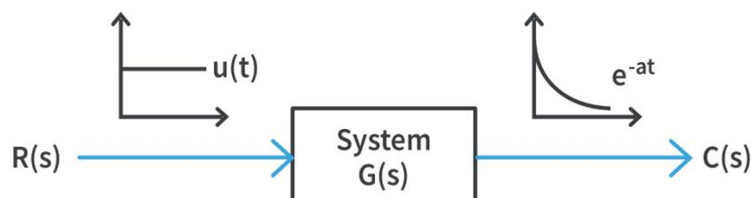
**Figure 4.1:** Illustrates the graphical presentation of transfer function.
