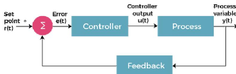
**Figure 1.3: Illustrates circuit diagram of closed-loop system.**
