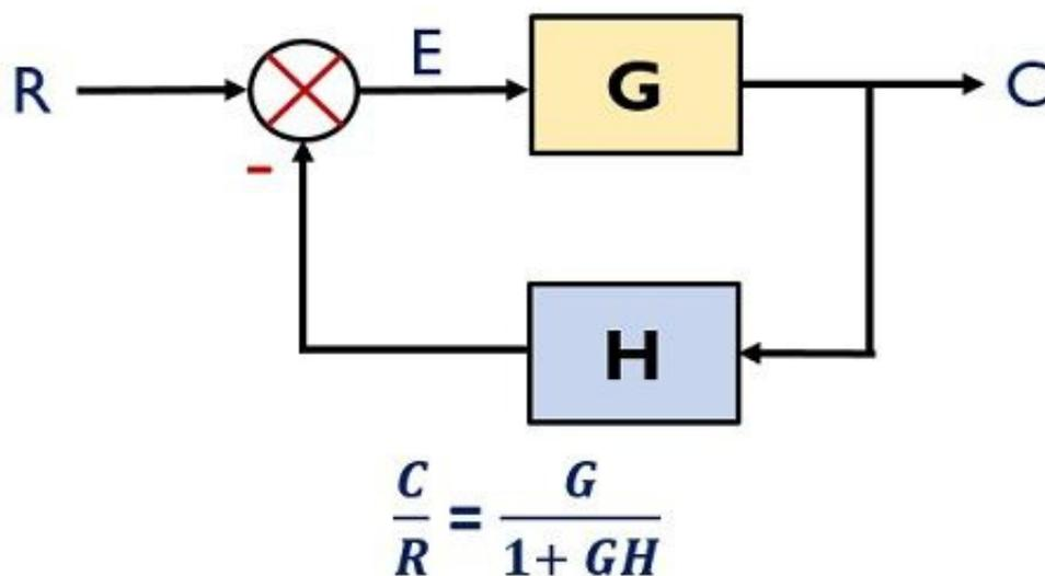
**Figure 1.7:** Illustrates the negative feedback loop with input output signal
