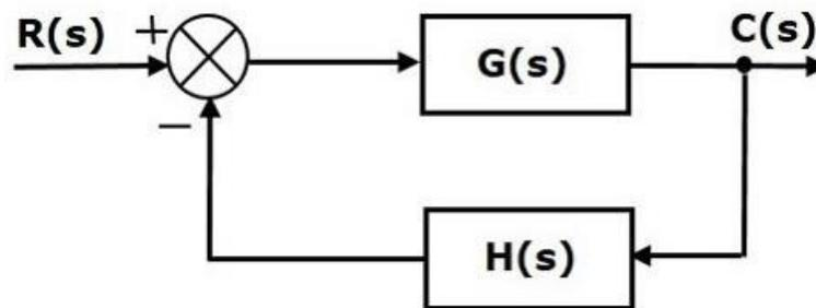
**Figure 9.3:** Illustrates the Block diagram of closed loop control system.
