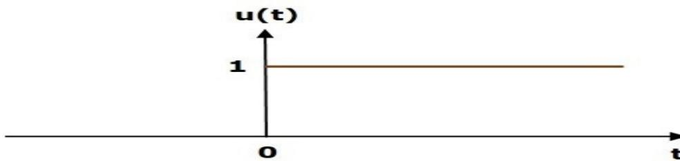
**Figure 8.5: Illustrates the unit step signal.**
