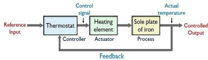
**Figure 2.3: Illustrates circuit diagram the automatic electric iron.**
