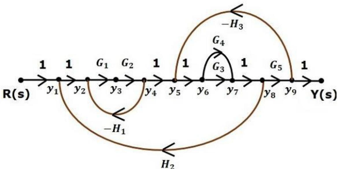
**Figure 7.6:** Illustrates the signal flow graph with their summing point.
