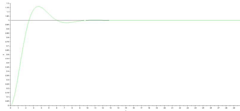
**Figure 6.6: Illustrates an open loop pole to a higher order system can make the system unstable.**
