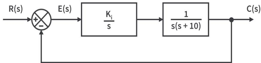
**Figure 6.10: Illustrates the Proportional-integral (PI) control effectively rejects the disturbance.**
