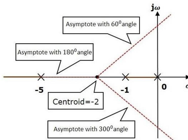
**Figure 10.3:** Illustrates the displays the centroid and three asymptotes.
