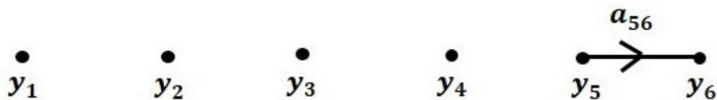
**Step 6** – Signal flow graph of overall system is shown in the following figure.
