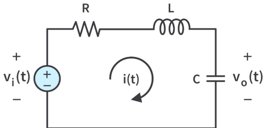
**Figure 7.2: Illustrates the circuit diagram of RLC.**
