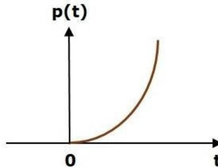
**Figure 8.7: Illustrates the unit parabolic signal with respect to time.**
