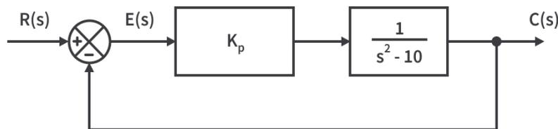
**Figure 6.13:** Illustrates the System instability lies inside the right half of the s-plane.
