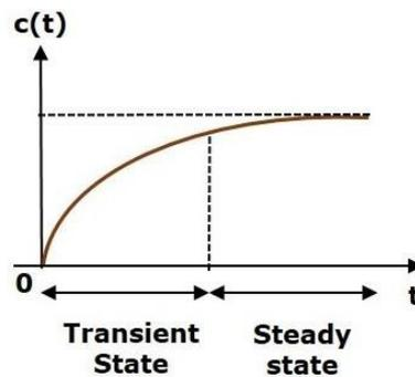
**Figure 8.4: Illustrates both the transient and the steady states.**
