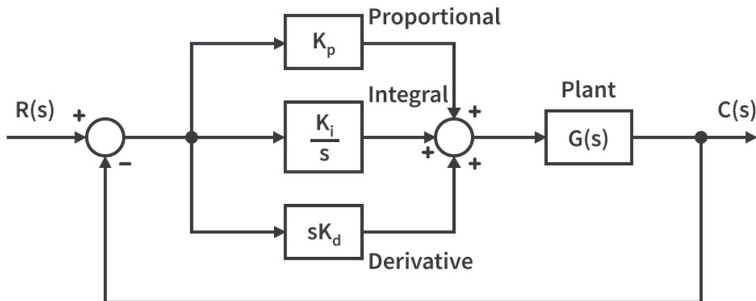
**Figure 6.1: Illustrates the block diagram of the system using PID control.**
