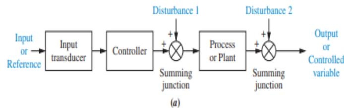
**Figure 2.5: Illustrates the configuration of open loop system.**
