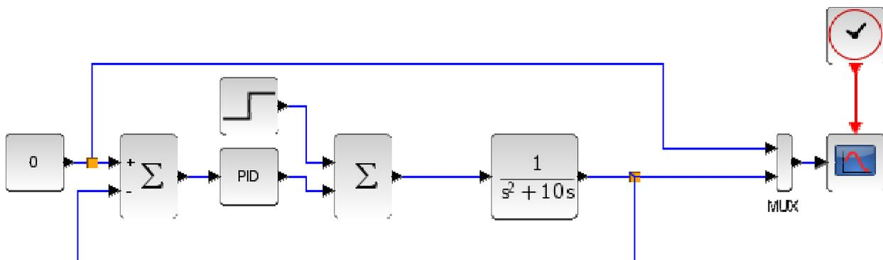
**Figure 6.8:** Illustrates the transfer function connecting the disturbance  $D(s)$  towards the output  $C(s)$ .
