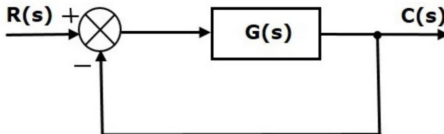
**Figure 9.2 Steady State Errors in Feedback Systems in Unity**
