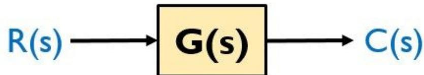
As we know that the transfer function of a system is specified as output by input. Thus for this system, it is given as:
