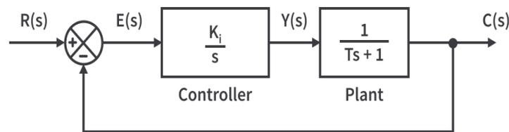
**Figure 6.5: Illustrates the Integral control does not address the immediate problem but rather the accumulated error.**
