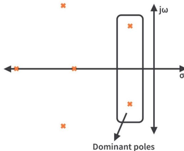
**Figure 7.1 illustration of a higher order system as well as its prominent poles**
