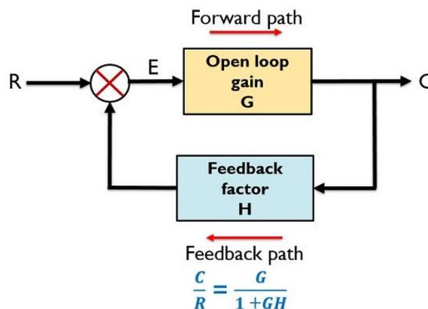
**Figure 1.5: Illustrates the control system with feedback.**
