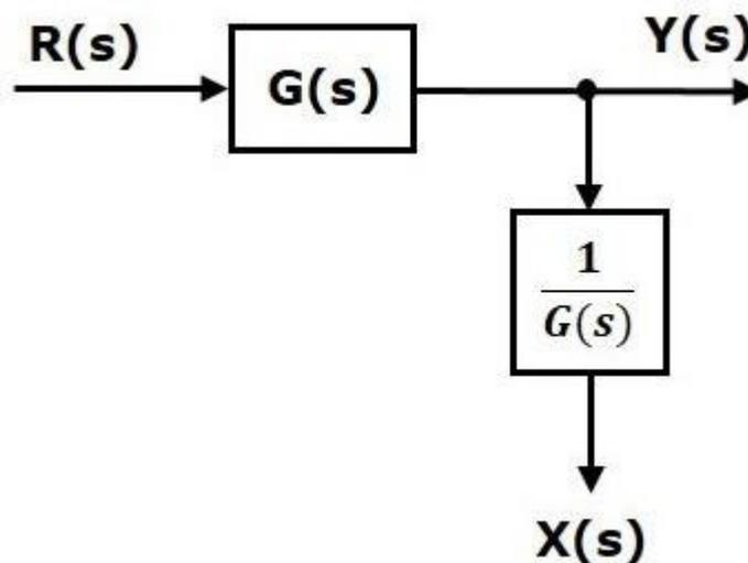
Changing the takeoff point from one that is after a blocks to one that is before the block. Take a look at the block diagram in the accompanying graphic. In this case, the takeoff point is after the block.
