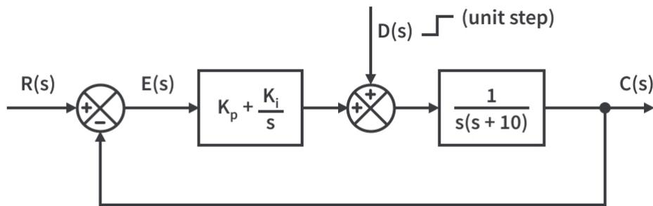
**Figure 6.9:** Illustrates the Combine proportional control plus integral control within the same system.
