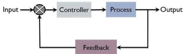
**Figure 1.10: Illustrates the closed-loop system is obtained by the output created by adopting a feedback route.**
