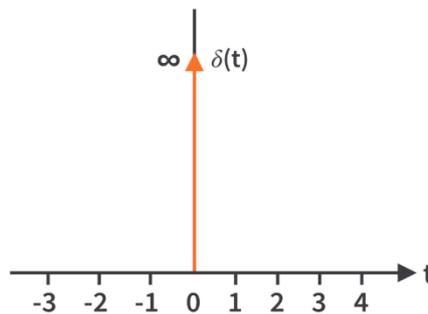
**Figure 4.3 time vs impulse signal**
