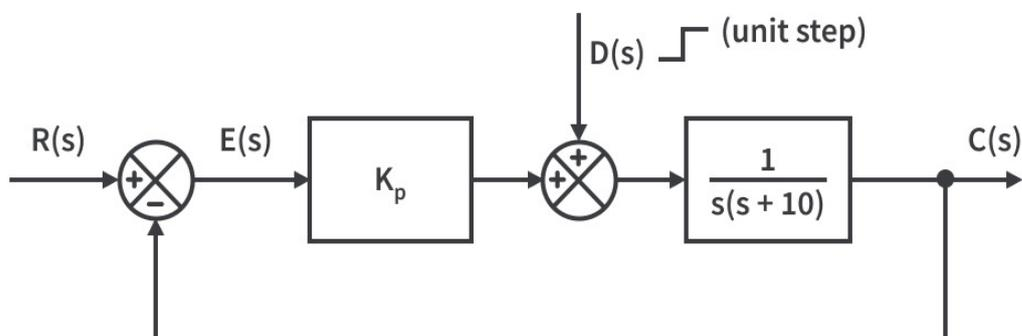
**Figure 6.7: Illustrates a block schematic of the system using proportional control and an external disturbance.**
