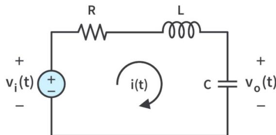
**Figure 4.5: Illustrates the circuit diagram of identifying the transfer function.**
