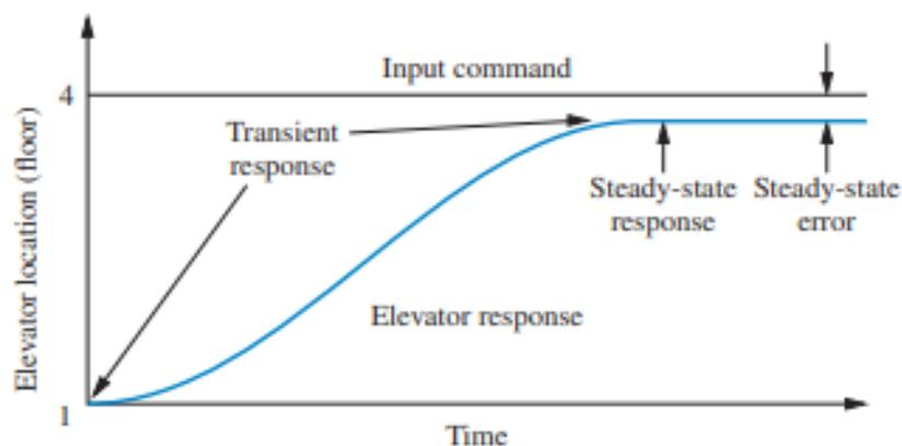
**Figure 2.4:** Illustrates the graphical representation of elevator versus time.
