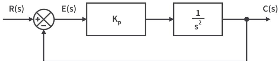
**Figure 6.11: Illustrates the aforementioned system's closed loop transfer function.**
