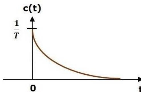
**Figure 8.8:** Illustrates the unit impulse response.
