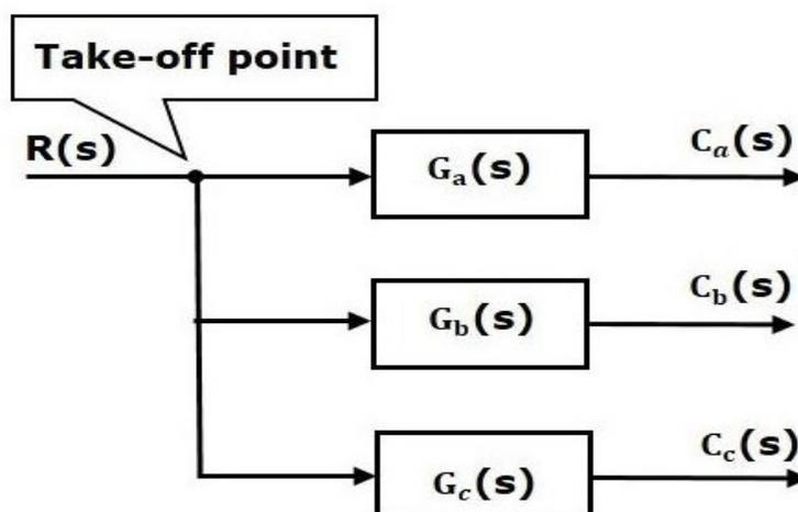
**Figure 5.4:** The take-off point is utilized in the following illustration to link the same input,  $R(s)$ , to two more blocks.
