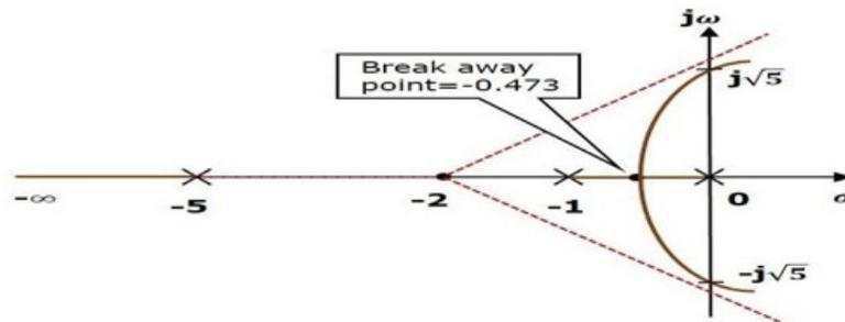
**Figure 10.4:** Illustrates the root locus diagram again for specified control system.
