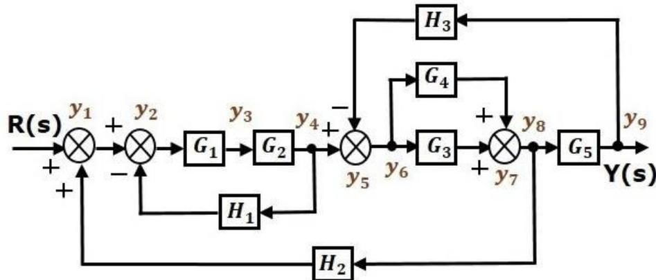
**Figure 7.5:** Illustrates the signal flow graph using the following block diagram.
