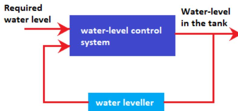
**Figure 1.4 water level control system**
