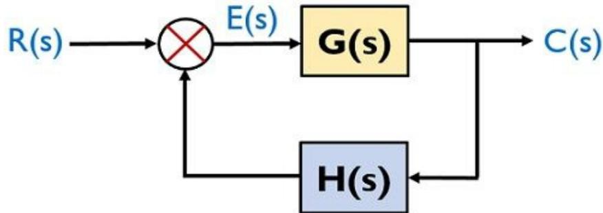
Figure 1.8: Illustrates the closed-loop control system.
