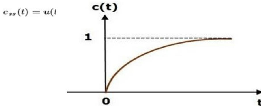
**Figure 8.9:** Illustrates the unit step reaction is shown in the accompanying.
