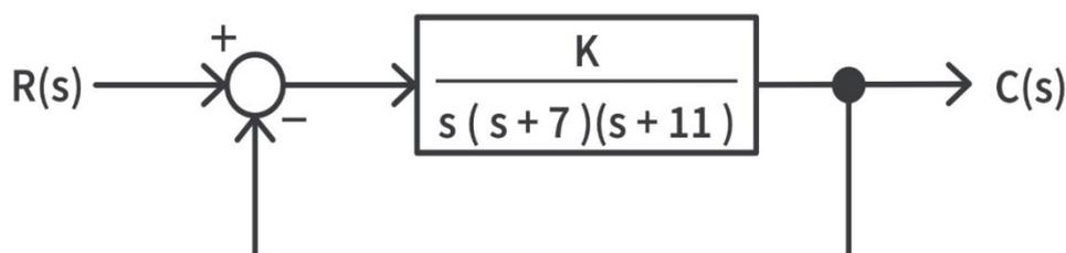
**Figure 7.3: Illustrates to consider the system with an open-loop transfer function.**
