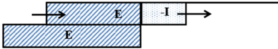
Figure 5.7: Illustrates the voltage is held by the source to the value E .
