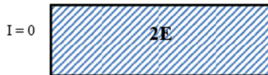
Figure 5.6: Illustrates the distribution along the whole line will be a voltage of 2E and a current of zero.
