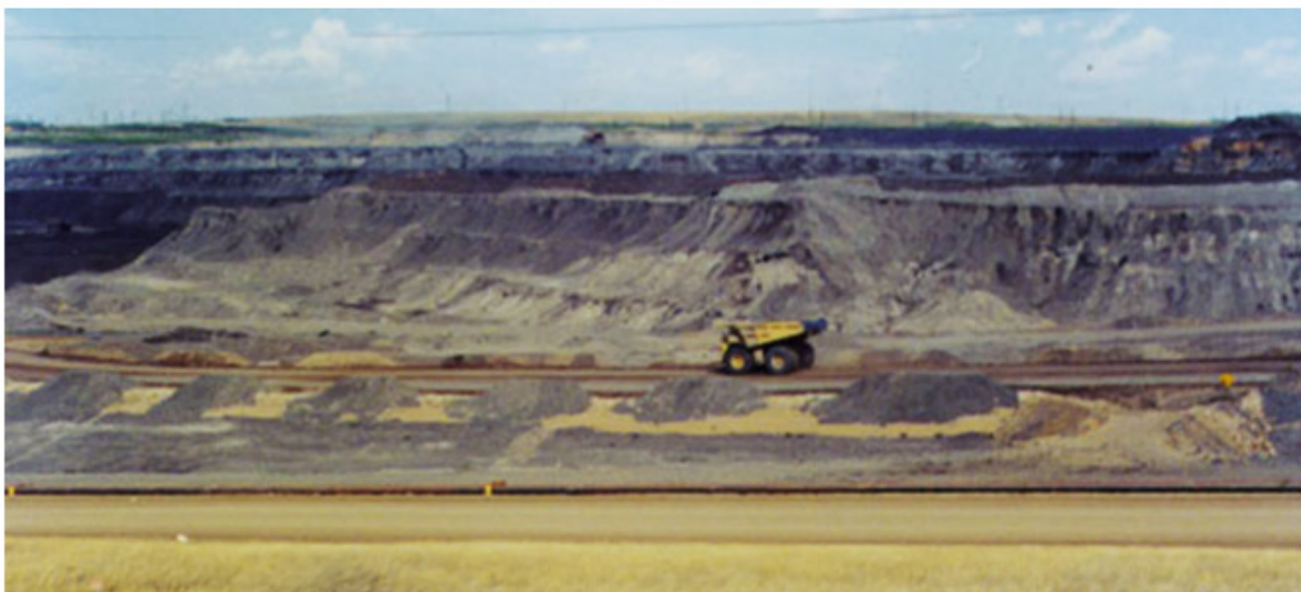
Figure 2: Athabasca tar sand. The oil-impregnated sand is mined and the heavy oil is separated from the sand with hot water.
