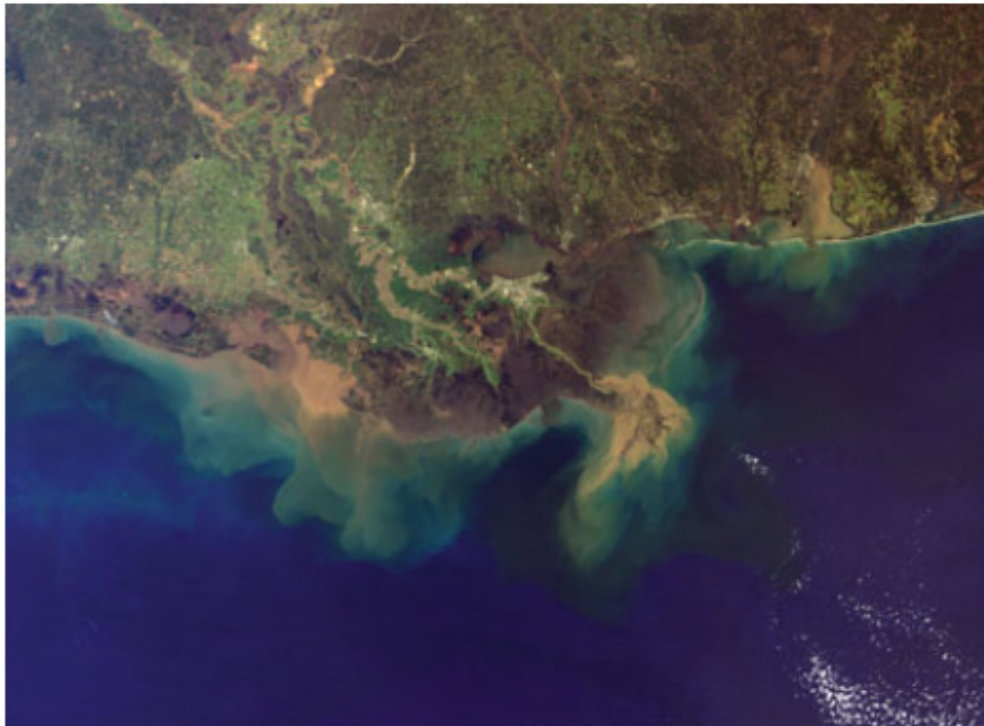
Figure 1: Satellite photograph showing the distribution of clay outside the Mississippi delta. The limited extent of the delta mud is due to flocculation of the clay particles when freshwater is mixed with ocean water.
